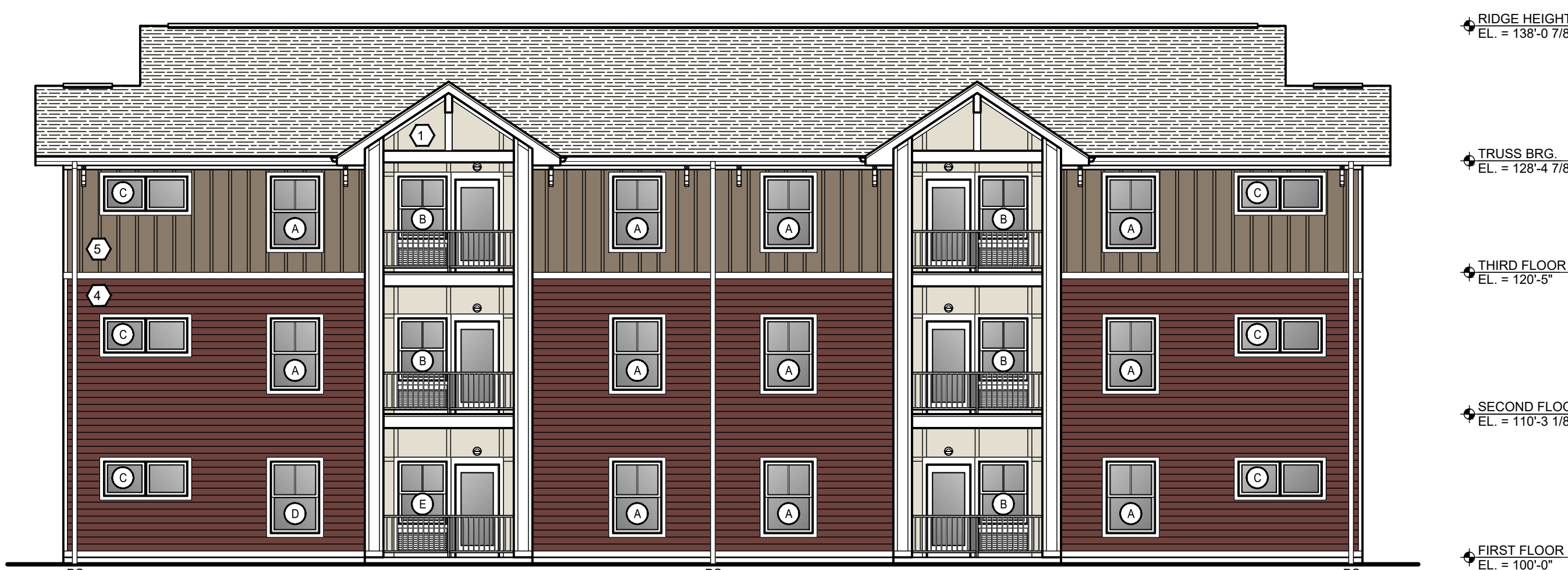
BUILDING #2 WEST ELEVATION SCALE: 1/8" = 1'-0"
