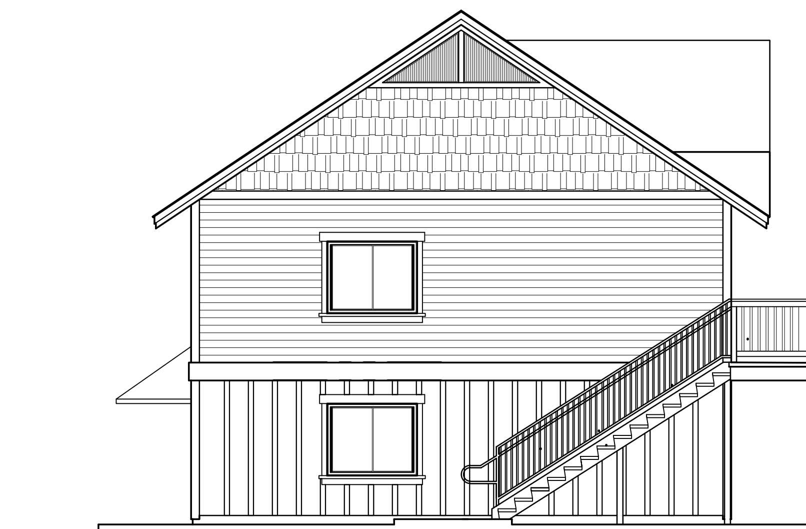
3 SIDE (EAST) ELEVATION - (Building 'A') SCALE: 3/16"=1'-0"
