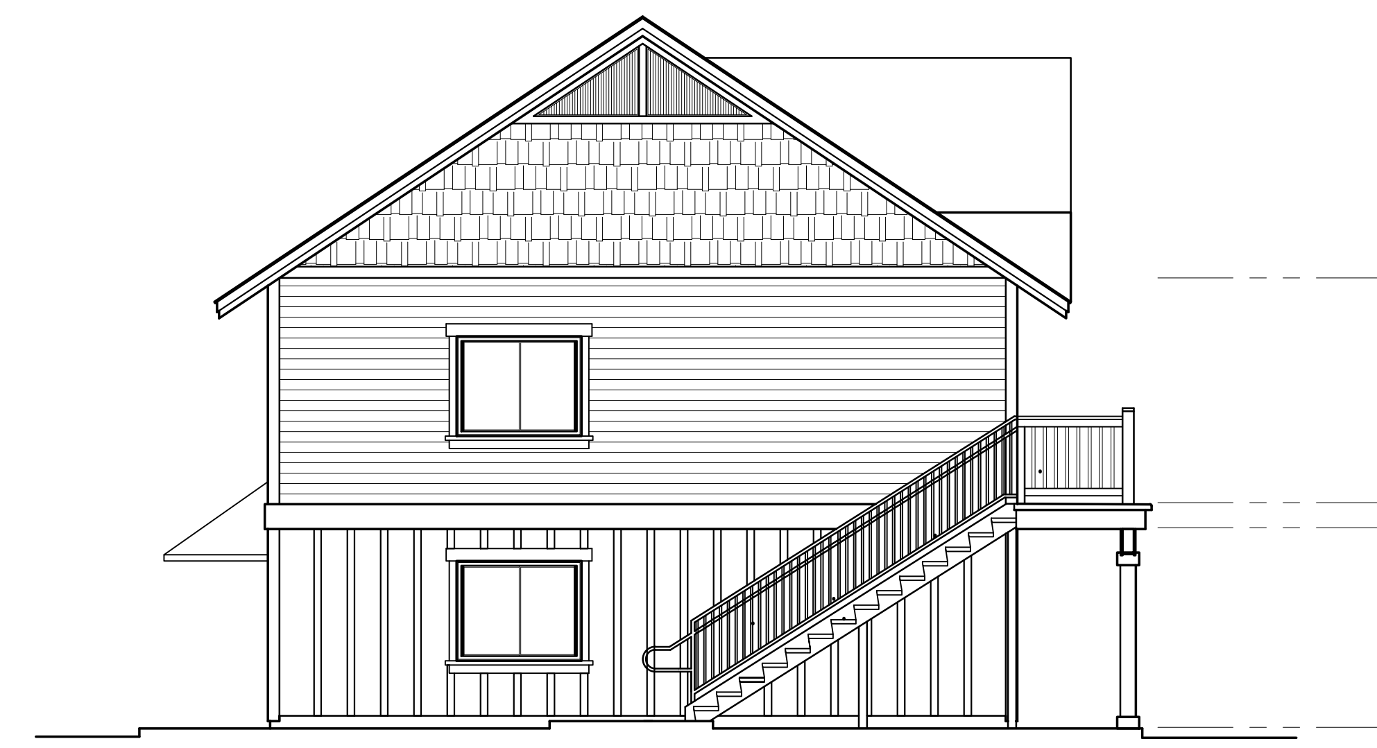
3 SIDE (EAST) ELEVATION - (Building 'A') SCALE: 3/16"=1'-0"
