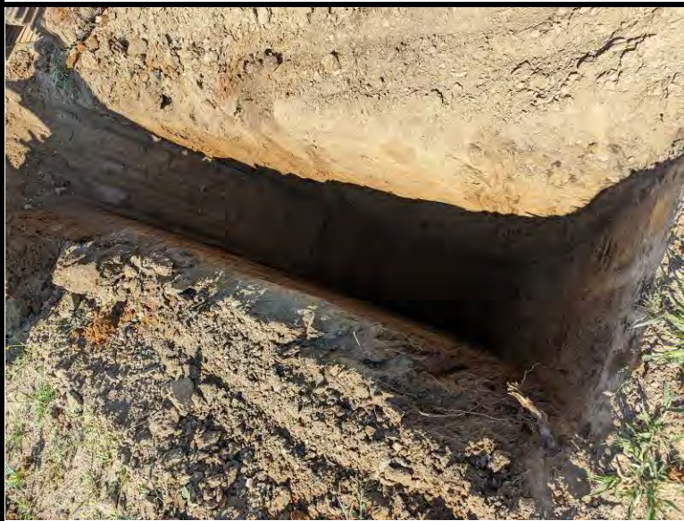
Subsurface soil profile within test-pit TP-2
