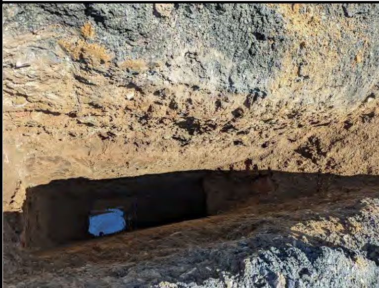
Subsurface soil profile within test-pit TP-8
